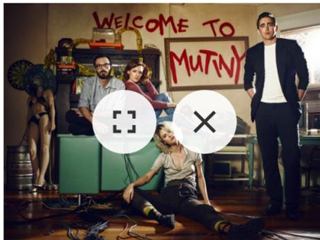
**Figure 5.14:** `keep-thumb` component: gets an image as argument and displays it with additional fullscreen and delete controls.
