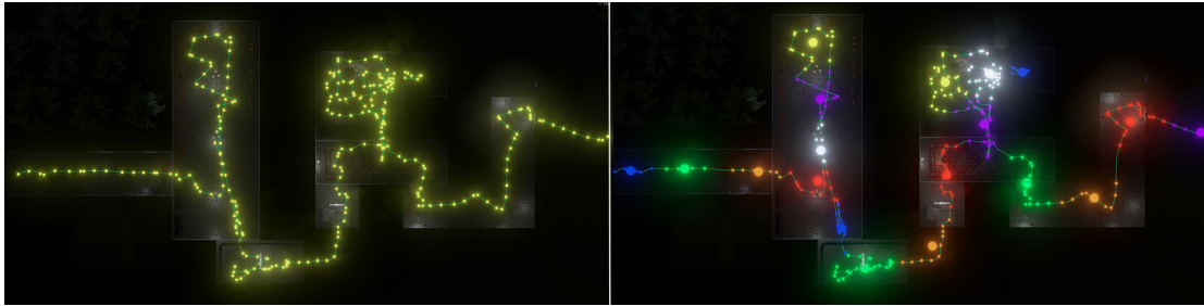
Figure 4.5: Left: Yellow circles resemble the paths point characteristics. Right: Characteristic points of the graph are grouped by spatial proximity. Color resembles which points belong to the same group. The big circle represents the centroid of a group.
