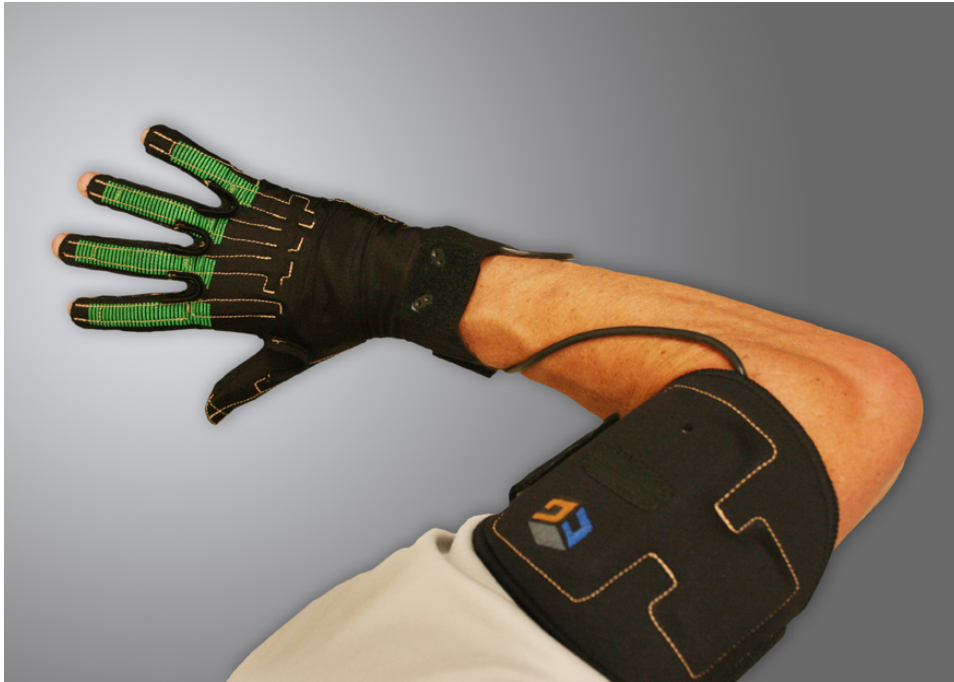
Figure 2.2: CyberGlove Model III data glove by CyberGlove Systems .
