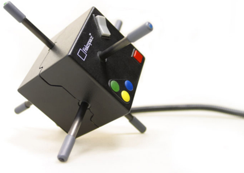
Figure 2.4: Cubic Mouse controller by Fröhlich et al.
