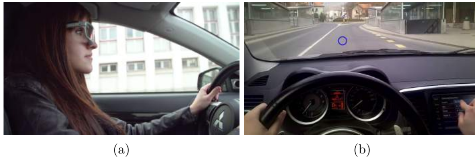
Figure 2.5: Driver performance capturing with eye tracking wearable [85].
