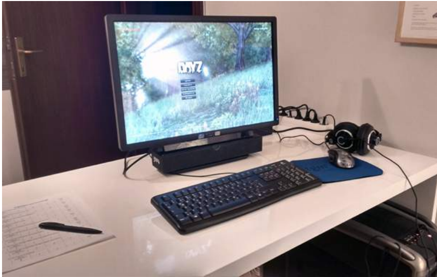
Figure 4.7: The setup consisting of a standard PC, keyboard and mouse, a Tobii EyeX Eyetracker and headphones.
