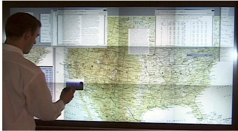
Figure 2.1: Post Brainstorm enables the user to work with high resolution images, application windows and hand drawn material. All interaction is performed using a digital pen that can also be used to sketch notes or take annotations. (Courtesy of François Guimbretière et al.)
