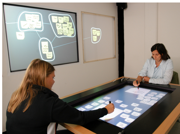
Figure 2.2: While table is used to write down ideas, the wall-display provides an overview over the existing ideas and enables structuring (Courtesy of Otmar Hilliges et. al).
