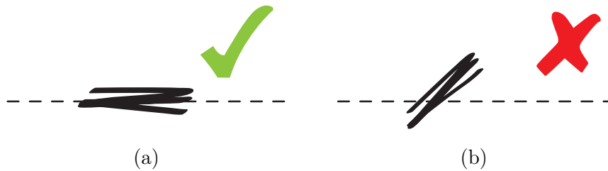
Figure 5.6: (a) The gesture is only recognized when the main direction is horizontally. (b) Otherwise the .NET GestureRecognizer does not identify the gesture as performed correctly.
