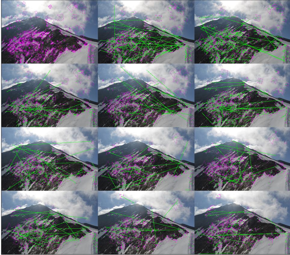
**Figure 4.5:** The sequence with the result of the first tracking iteration. The SIFT features are in magenta, the green lines indicate the position of a feature in the previous frame.
