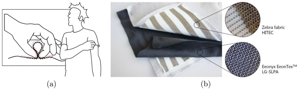
**Figure 2.2:** The use of the *Pinstripe* prototype (a) is illustrated and the composition of the *Flexiles* sensor (b) is shown. The illustration in (a) is taken from [10] and the image in (b) is taken from [21].
