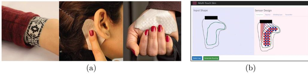
**Figure 2.3:** The flexible sensor can be placed on various body parts (a). A web application helps designers to create sensor layouts (b). The images are taken from [18].
