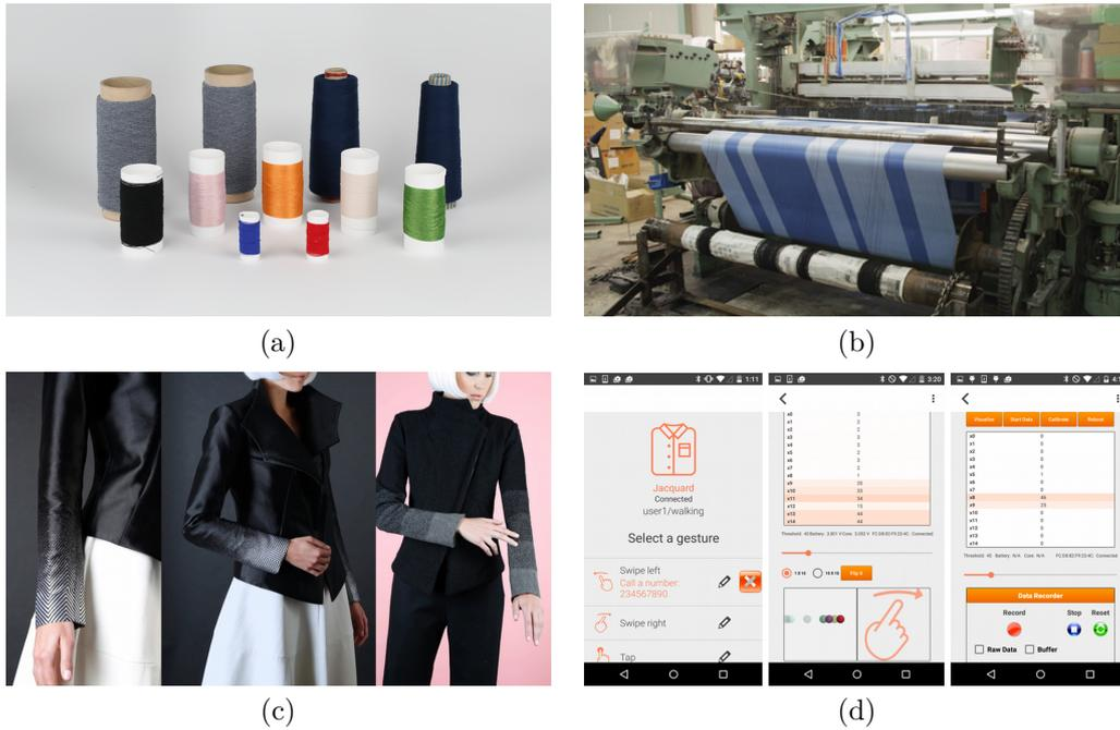
**Figure 2.1:** The yarns (a) developed in *Project Jacquard* can be used for weaving smart textiles (b) and were for example woven into the sleeve of a jacket (c). The developed mobile application is shown in (d). Images are taken from [23].
