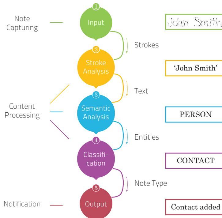
**Figure 5.3:** The technical structure of *PECAN* starts with the digital pen input (1), the handwriting analysis (2), a semantic processing (3), note classification (4), and ends with an output window displaying all analyzed contents (5).
