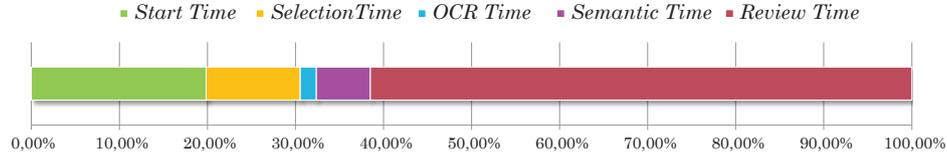
**Figure 7.8:** The average trial completion time for the adding phase of the *PECAN* Workflow was 17.8 seconds. 3.5 seconds (19.84%) were trial starting time until the content selection, 1.9 seconds (5.54%) selection time, 0.3 seconds (1.82%) handwriting recognition time, 1.1 seconds (6.13%) semantic analysis time and 10.9 seconds (61.51%) content review time.
