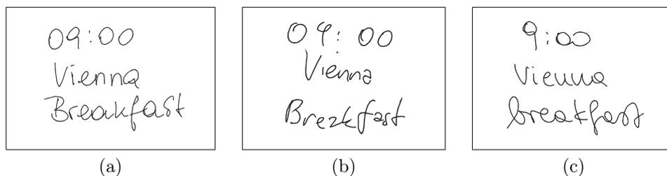
**Figure 7.1:** Handwriting examples (a) Participant 15: 0.0% errors, overall error rate for all notes  $M=1.33\%$ , (b) Participant 4: 5.00% error rate ('9' was recognized as a '4'), overall error rate for all notes  $M=6.33\%$ , (c) Participant 5: 15.00% error rate (no leading '0', and Vienna was recognized as 'Vieuua'), overall error rate for all notes  $M=8.87\%$ .
