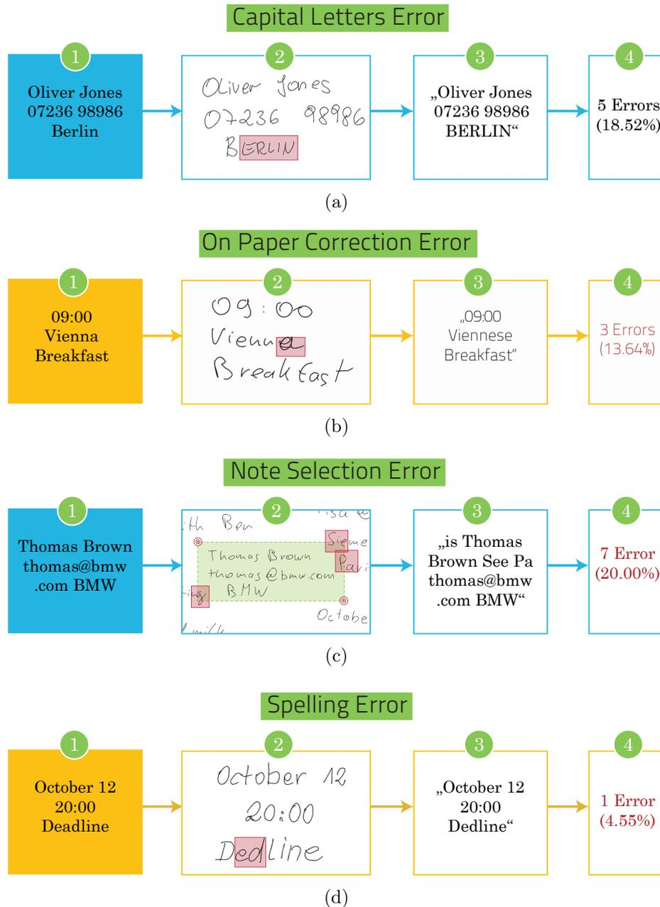
**Figure 7.2:** A visualization of the error categories: (1) shows the template text, (2) the actual written text by the participant, the error that has occurred is marked in red, (3) the text analysis result by the handwriting recognizer, (4) Minimum String Distance (MSD) error calculation (error percentage).
