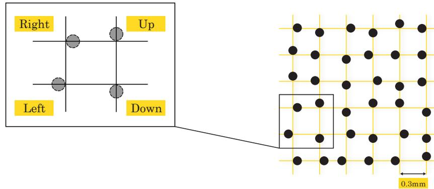
**Figure 5.2:** The Anoto pattern is a proprietary pattern to identify correctly the current location of the pen. It consists of small dots with a diameter of 0.1 mm. Through displacement of the dots along the square grid, a unique non-repetitive pattern is created.
