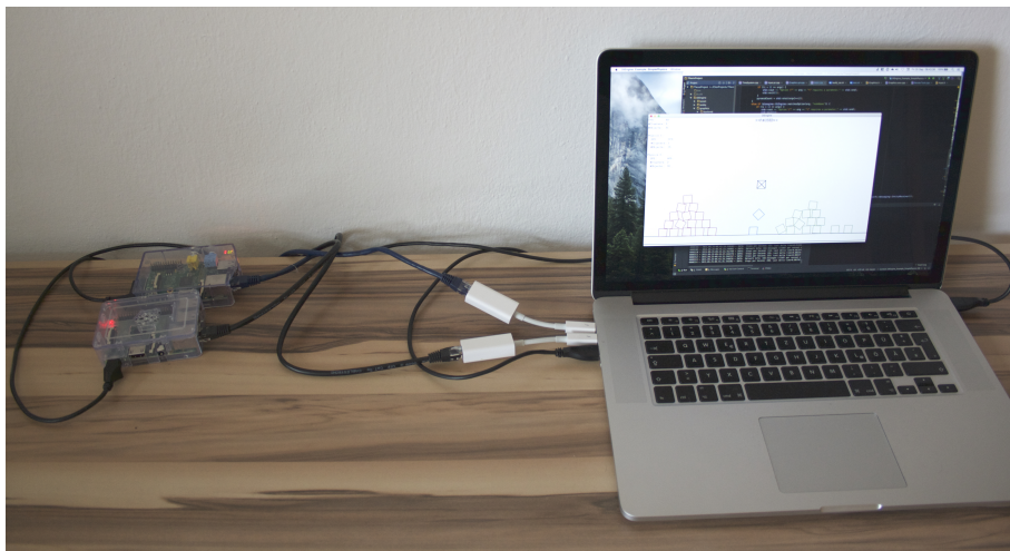
Figure 4.1: Example hardware setup running a test configuration. In this case the notebook running OS X also acts as network switch and via USB as power source for the Raspberry Pis .
