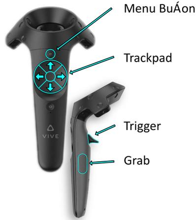
**Figure 4.2:** The input options of the HTC Vive motion controller.
