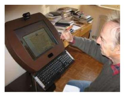
Figure 3.1: Picture of the final *Mobitable* [13, p. 847]. The touch screen is slanted to ease the use. A camera is placed on the top facing the user and a keyboard underneath.
