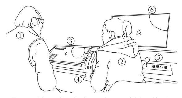
**Figure 4.6:** A diagram of the technical setup. 1: the navigator (elderly people); 2: the captain (research staff); 3: 24 inch touchscreen of the navigator; 4: Pro Flight Throttle Quadrant for variant C; 5: arcade game controller for the captain; 6: 55 inch screen for both players.
