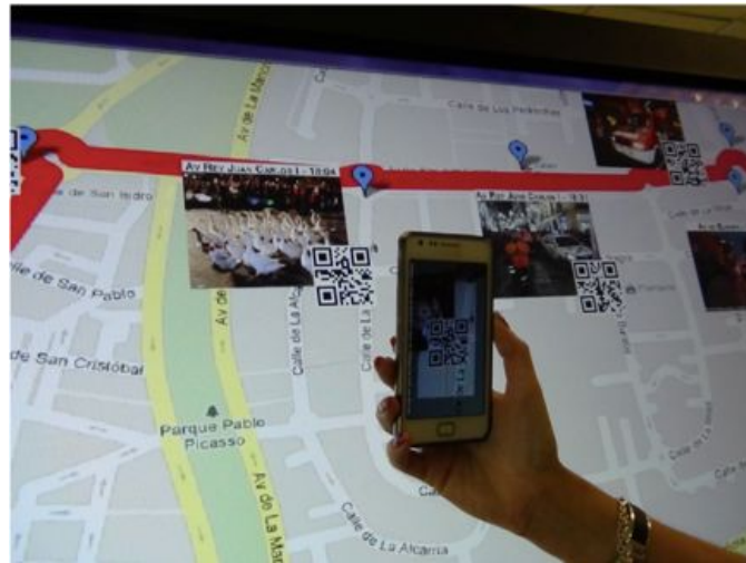
Figure 2.1: The setup in [8] consisted of a shared display and multiple mobile devices. Additional information to the interaction points can be gained by scanning QR-Codes.
