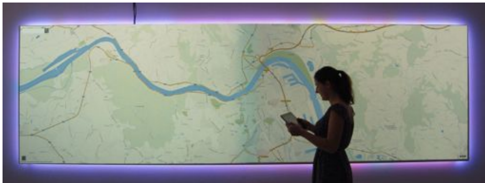
Figure 3.1: The basic setup consists of a digital whiteboard and gets extended with an additional tablet computer for every user.
