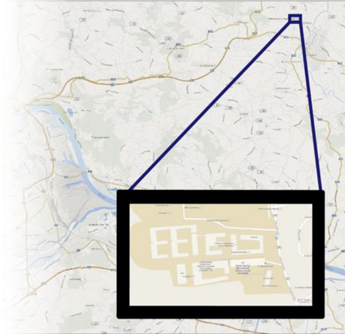
Figure 3.5: If the tablet's view is zoomed-in and the whiteboards current zoom level is very low, a rectangle representing the current tablet's view is hard to detect. Therefore, rendering multiple, magnified rectangles is important.
