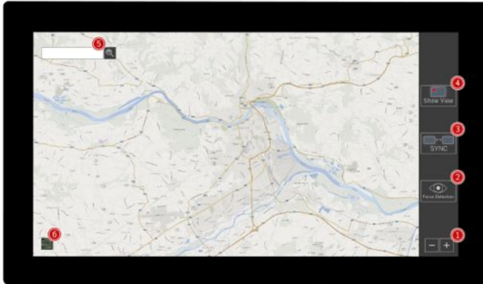
Figure 3.3: The tablet application. On the right border of the display is the button bar with the Show View - (4), the Sync - (3), the Focus Detection - (2) and the Zoom -buttons (1). In the top and bottom corners on the left, are a search box (5) and a button to change the map view's type from hybrid to satellite (6).
