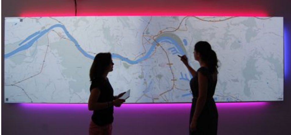
Figure 3.12: The ambient light can show off-screen visual cues for multiple users simultaneously.
