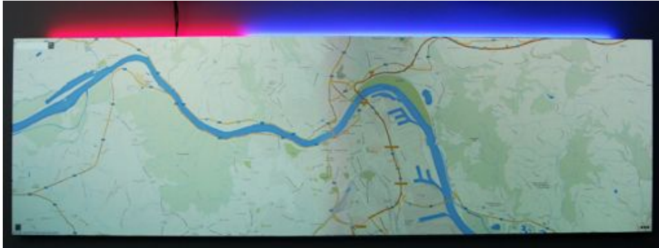
Figure 5.9: When two borderlines overlap, the RGB values for the appropriate leds are overwritten by the device, which sends the Show View -event later.
