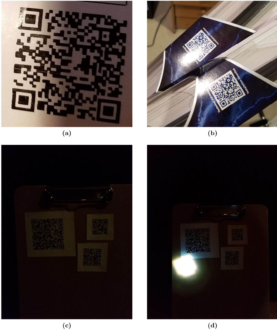
Figure 2.8: Examples of QR codes with flawed lighting conditions.
