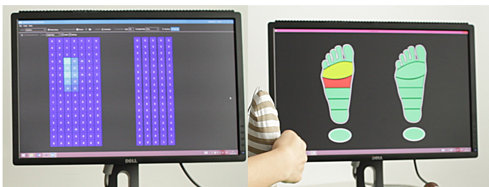
Figure 4.9: Software visualizations of pressure readings from the proCover sock. Individual sensing intersections from the sock are visualized using software developed in PyzoFlex [19] (left). Sensing intersections are grouped into distinct sensing regions along the bottom and top of the foot, as well as the ankle. Warmer colours indicate higher pressure readings (right).
