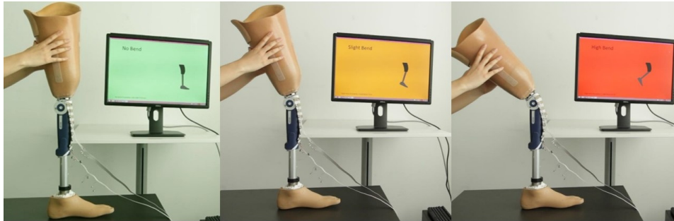
Figure 7.5: The final prototype of the sensing knee guard. Mounted on a prosthesis, it can provide an approximation of the amount of bending in the leg in degrees. A visual representation of the amount of bending registered by the system is displayed using an on-screen graphic of a prosthetic leg.
