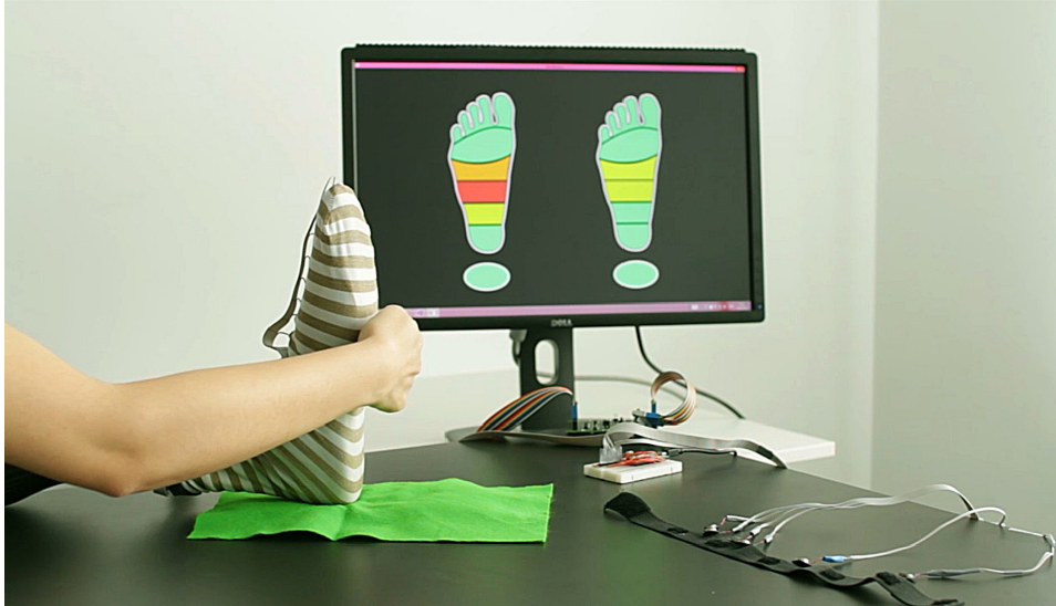
Figure 4.1: The sensing sock prototype consisted of a fabric-based sock and vibration armband driven by independent microcontrollers.
