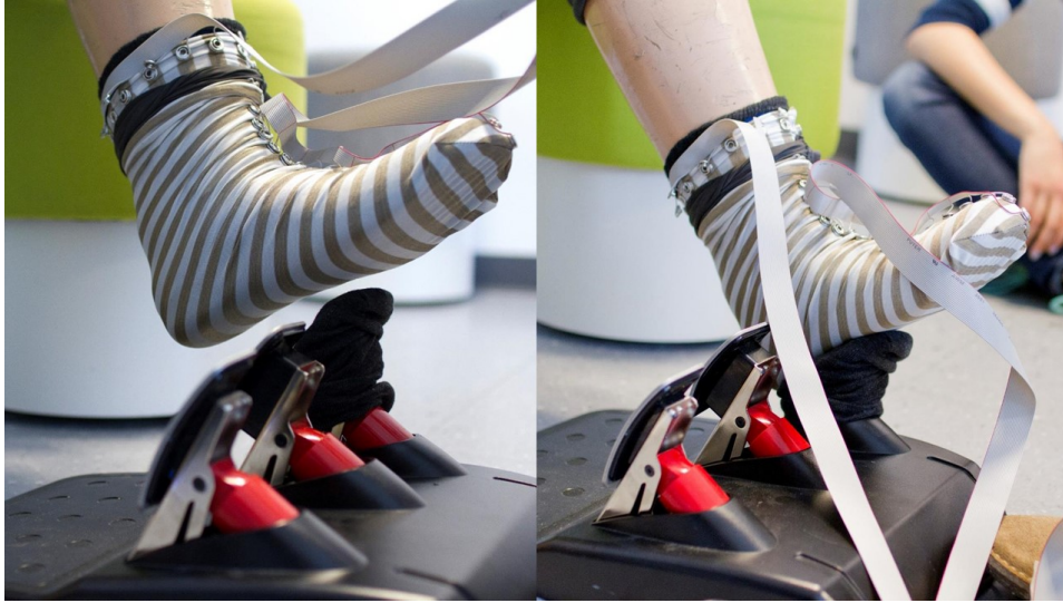
Figure 8.3: Each participant wore the sensing sock over his/her prosthetic leg and wore the vibration haptic feedback band on his/her right arm. The haptic feedback band was adjusted for each participant to fit snugly around the arm. With their eyes closed, participants were instructed to depress a car pedal to one of three different levels (shallow, medium, full). The number of times they could correctly perform each press was logged.
