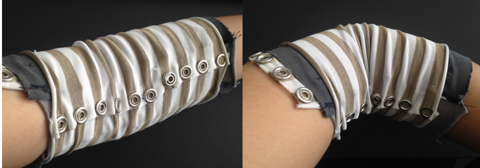
Figure 7.6: The full-sleeve prototype in an unbent (left) and bent (right) state. This design presents a risk for conductive lines to come together and electrically short one another on the concave side of the joint, as can be seen in the bent state. A half-sleeve form factor eliminates this risk.
