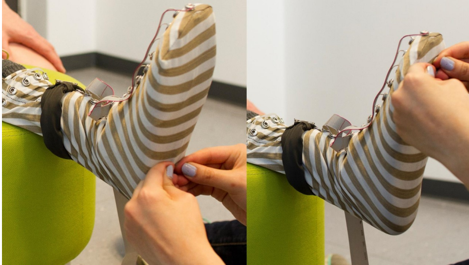
Figure 8.2: Each participant wore the sensing sock over his/her prosthetic leg, and each wore the vibration haptic feedback band snugly around his/her right arm. With their eyes closed, participants were asked to report whether the ball or heel of their prosthetic foot was being pressed. The number of correct answers were logged for each condition (with sock, without sock).
