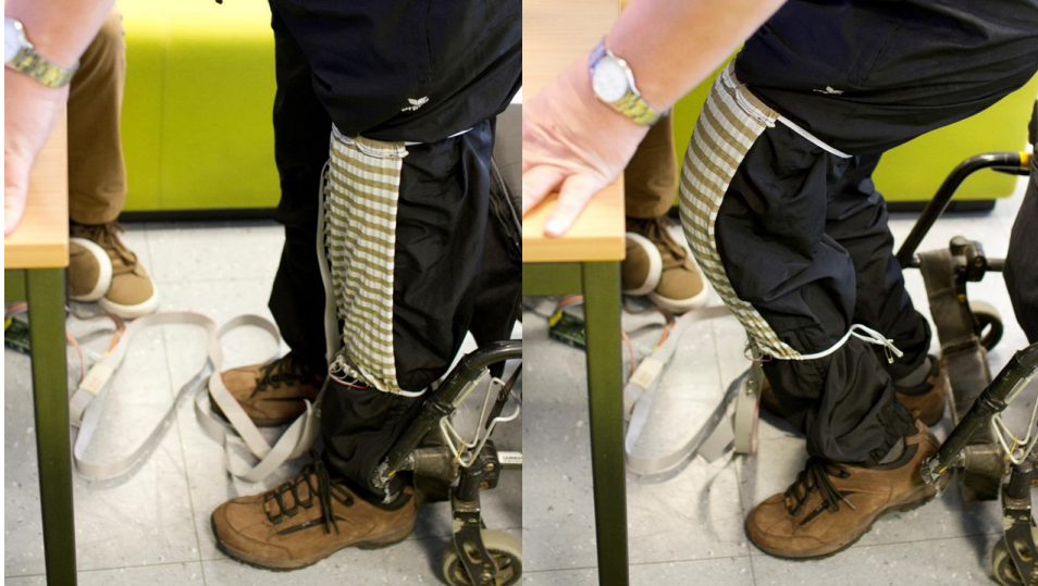
Figure 8.4: Two participants, each with an above-knee amputation, were asked to bend their prosthetic legs to three different degrees (no bend, slight bend, high bend) with the knee guard strapped over the knee-joint of their respective legs. The system was trained for each individual, and the number of times the trained system could correctly classify the true bend-state of the leg in test trials was logged.
