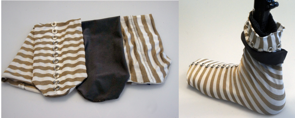
Figure 4.7: Three textile layers (left) come together to form the proCover sensing sock prototype (right).
