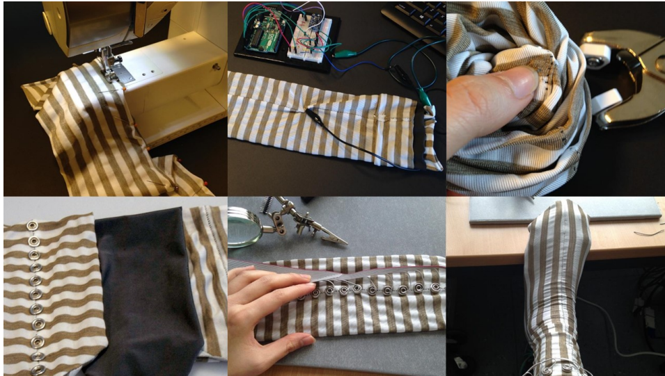
Figure 4.6: Process shots from making the sock. A sheet of zebra fabric is being sewn into a sock using a sewing machine (top-left); a single sensing intersection is hooked up for testing its change in resistance under pressure (top-middle); female snap fasteners are attached to each conductive line on a sock (top-right); the three layers are ready (bottom-left); male-snap fasteners are soldered to the ends of each wire in a ribbon cable (bottom-middle); a column-sock with wires attached to the sock via snap fastener connections (bottom-right).
