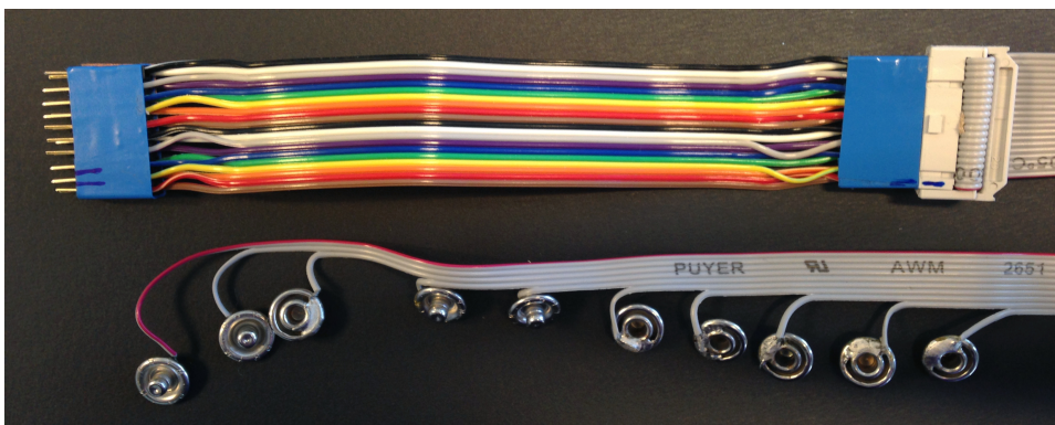
Figure 4.4: Electrical connectors. Male snap fasteners, soldered to the ends of ribbon cable, are used to connect the fabric to the measurement hardware.
