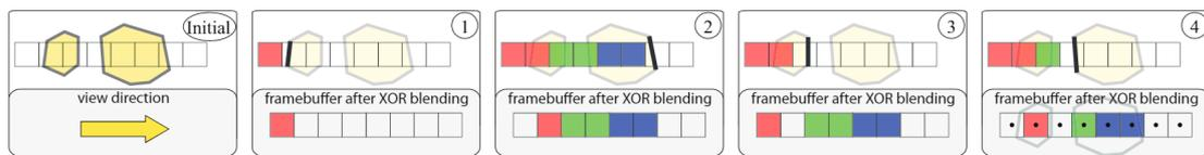
**Figure 2.4:** This image demonstrates the voxelization technique using a simplified example. The bitmask creation, as well as the combination process of those masks, is shown. Source: [7].
