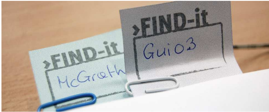
Figure 3.4: Two Find-it sticky notes for interactive bookmarking. Once a search request matches a keyword written on the Post-it note, the sticky note provides active feedback to the user by a constant wiggling motion.
