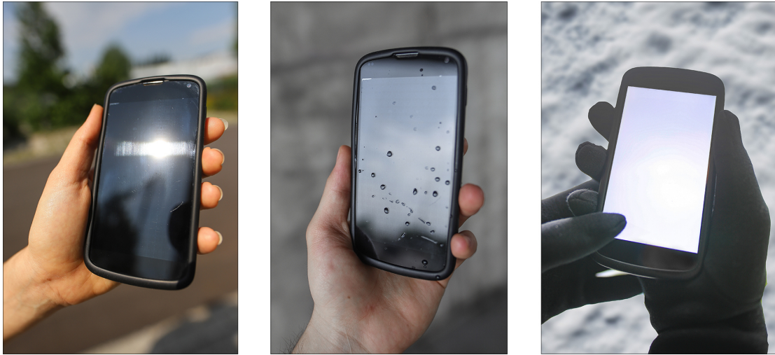
Figure 4.6: Influence of weather conditions on smartphone interaction. From left to right: strong sunlight, rain, and snow (user wearing gloves).
