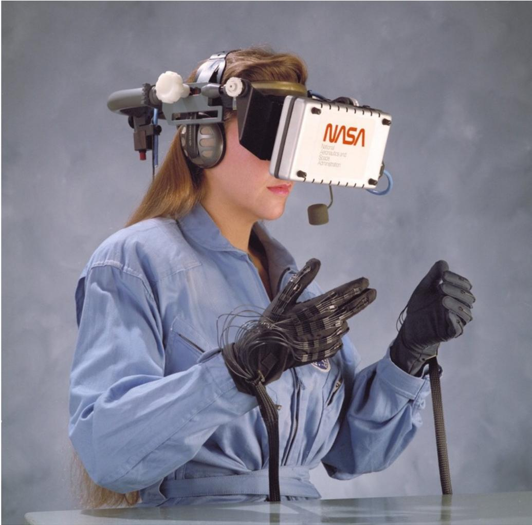
**Figure 2.2:** A later iteration of NASA's *Virtual Environment Station* including the tracked HMD and the tracked glove-like input devices.
