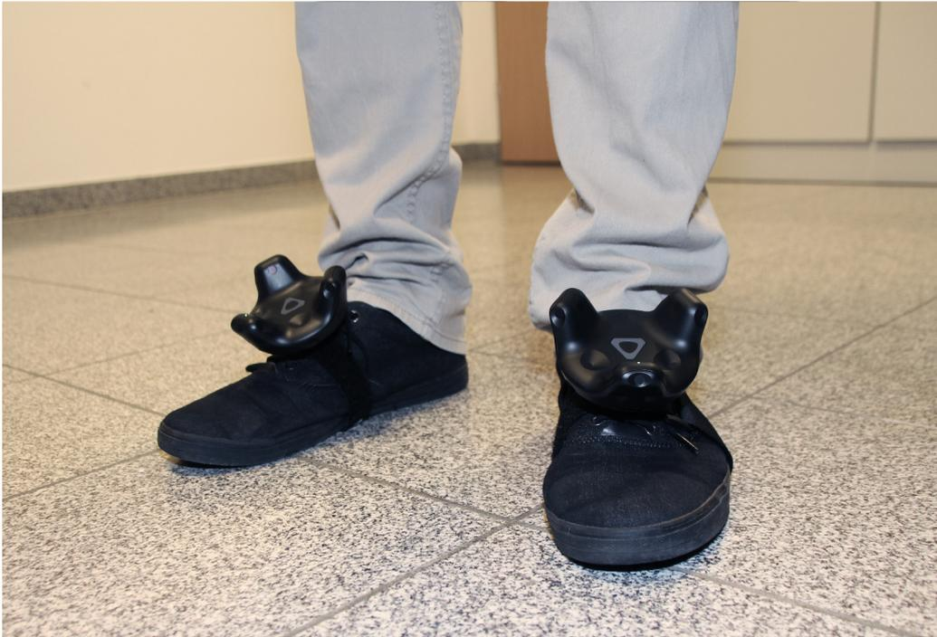
**Figure 6.2:** This is how the 6DoF trackers were attached to the user's and the interviewer's feet.
