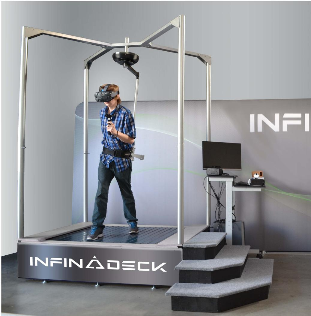
**Figure 2.5:** *Infinadeck* is an omnidirectional treadmill. It reacts to users' movements and keeps them in the center.
