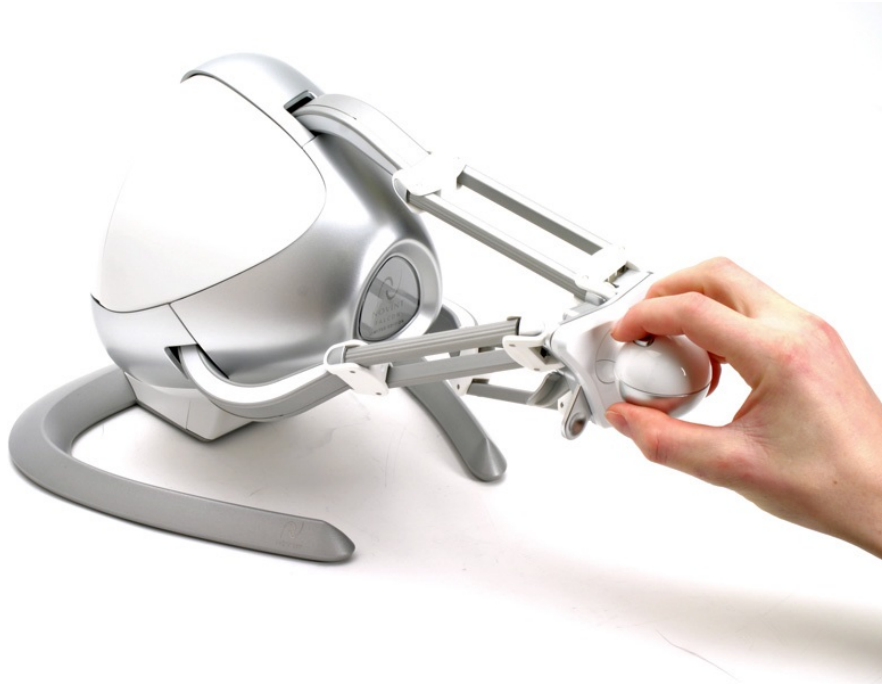
Figure 2.2: The “Novint Falcon” emulates haptic feedback. A user can control a 3D cursor inside the virtual environment.
