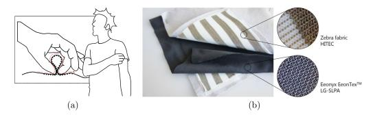
**Figure 2.2:** The use of the *Pinstripe* prototype (a) is illustrated and the composition of the *Flextiles* sensor (b) is shown. The illustration in (a) is taken from [10] and the image in (b) is taken from [21].
