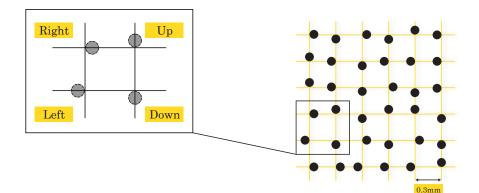
Figure 5.2: The Anoto pattern is a proprietary pattern to identify correctly the current location of the pen. It consists of small dots with a diameter of 0.1 mm. Through displacement of the dots along the square grid, a unique non-repetitive pattern is created.
