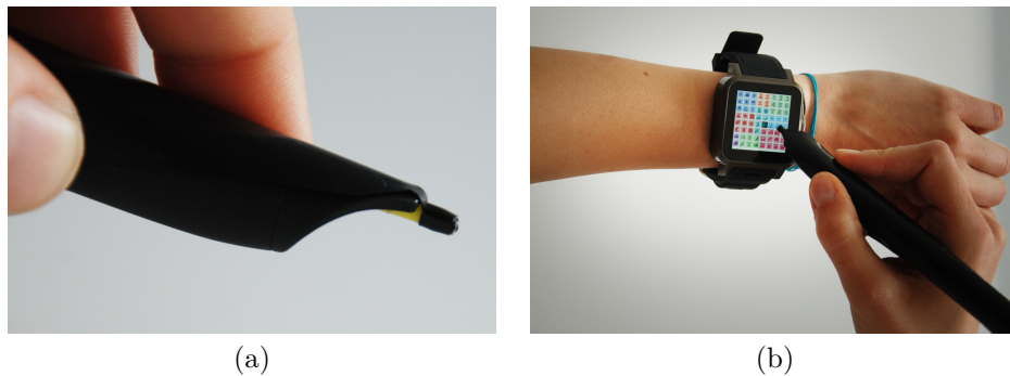
Figure 4.3: Polystyrene cover prototype detail view (a) and used with Pen Pen (b).
