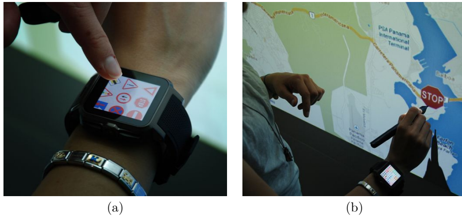
Figure 4.5: Combining whiteboard with smartwatch: Selection item on smartwatch (a) and insert item on whiteboard (b).
