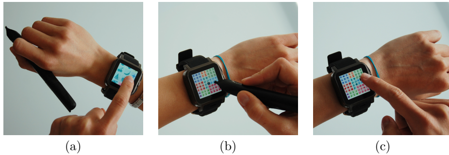
Figure 5.2: Techniques for combined use of the smartwatch and whiteboard: Bimanual Pen Touch (a), Pen Pen (b) and Pen Touch (c).
