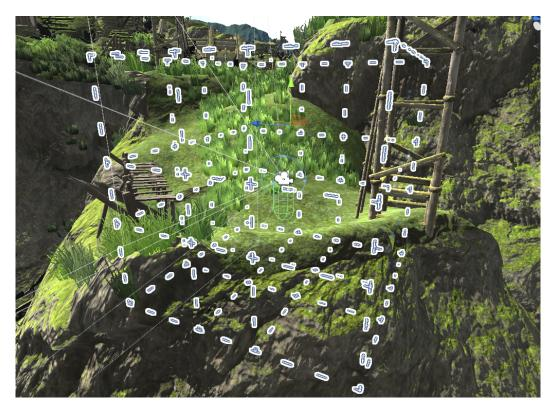
**Figure 3.4:** The capsule with the camera on top represents the player and their collider. The white frame is the aforementioned RF and its rotation is locked to the player-collider. The picture was edited to make the frame have thicker lines for better visibility and does not represent what the player sees.
