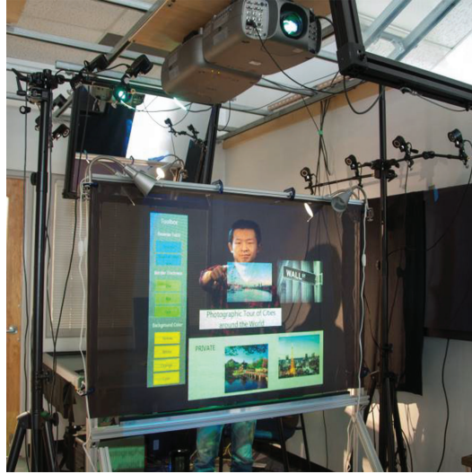
Figure 2.1: The two-sided transparent display allows for face-to-face collaboration. Image source [43].
