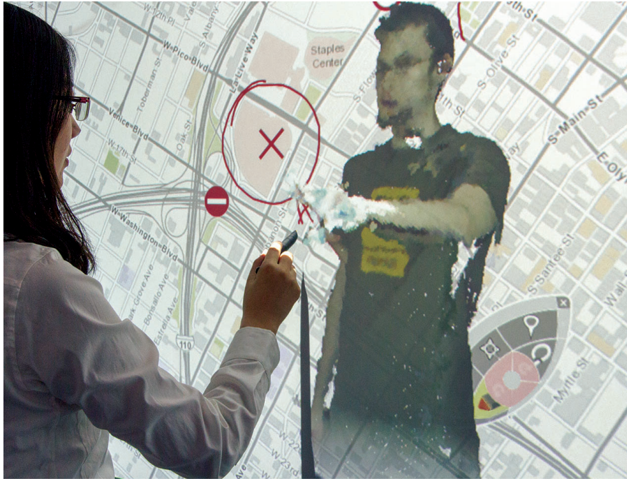
Figure 1.1: 3D-Board blends the virtual 3D embodiment of the remote user with the digital content of the interactive whiteboard.
