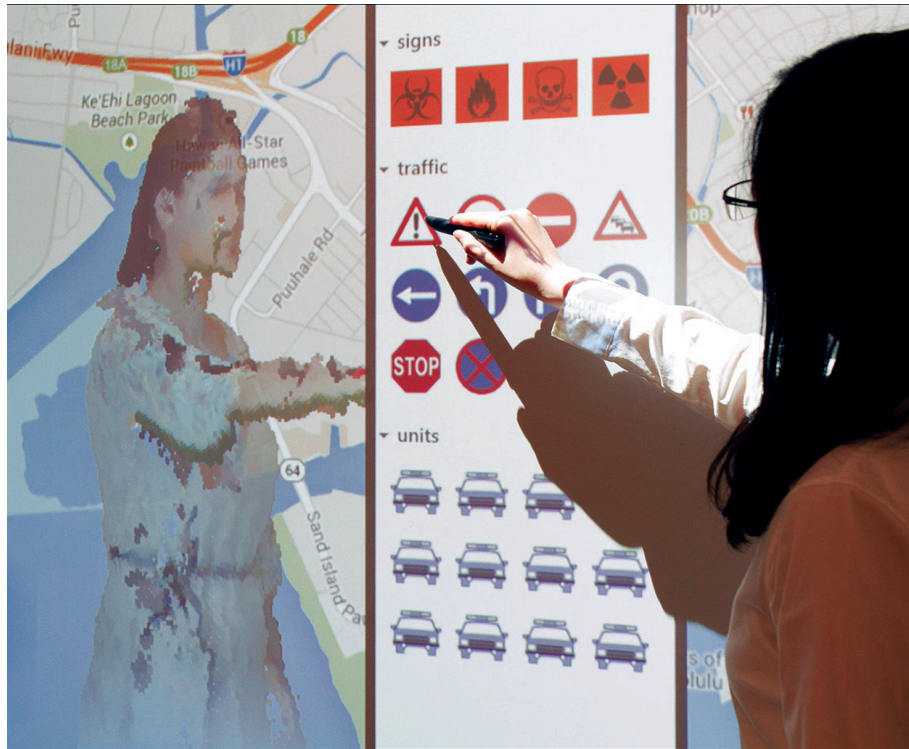
Figure 4.3: 3D-Board can be used to collaboratively keep track of crucial operational information. To increase the social presence of the remote user, the virtual embodiment is superimposed on top of the shared content, while important elements are not occluded.
