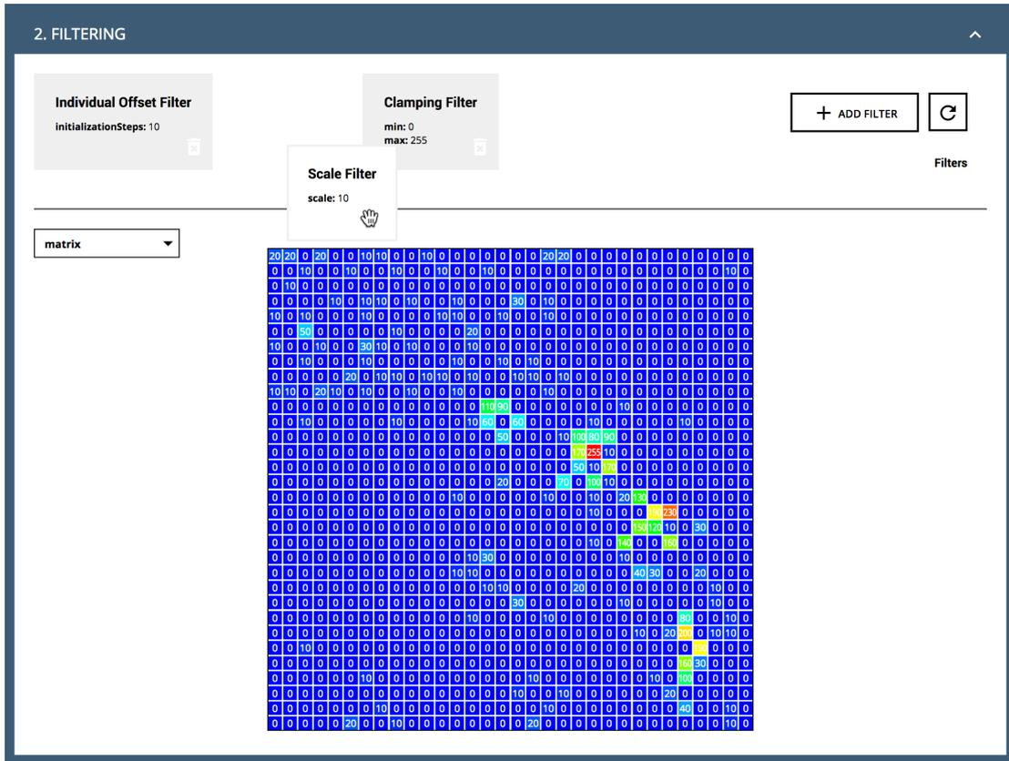
**Figure 5.2:** The second section allows to define new filters, delete existing filters or reorder the filters contained in the filter pipeline with a simple drag and drop mechanism. It also contains the visualization of the sensor data.
