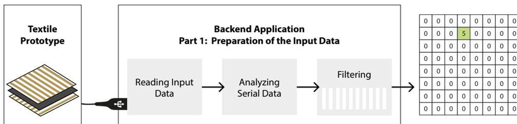
**Figure 3.2:** Data from the smart textile sensor is transmitted via a serial port. The first steps are to read the data from the serial port, analyze the input stream and transform the data to flattened arrays and apply filtering.
