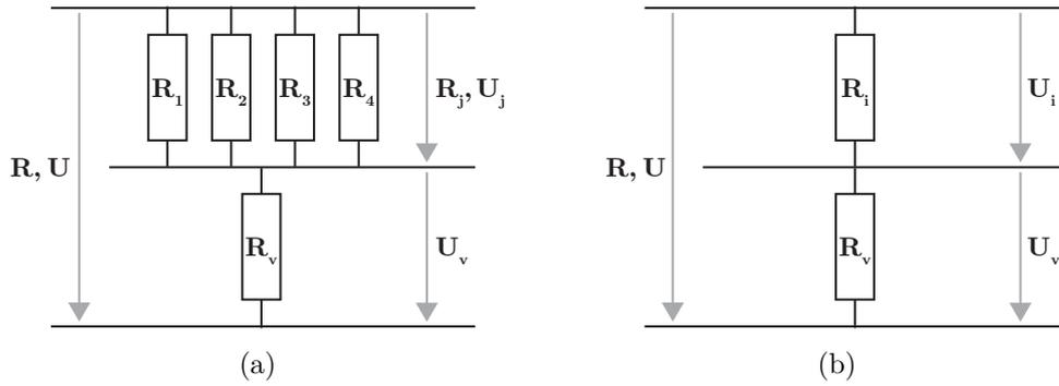
**Figure 6.5:** While all resistors (crosspoints of conductive yarns) of a specified sensor region  $R_j = (R_1, R_2, \dots, R_n)$  are connected in parallel,  $R_j$  is connected serially to a pull-down resistor  $R_v = 5.65 \text{ k}\Omega$  (a). The equivalent for a single sensor is shown in (b).
