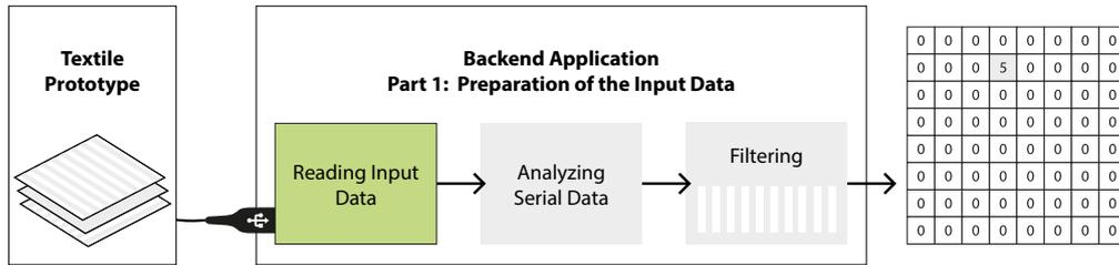
**Figure 4.1:** The first module handles reading the input data from the serial port.
