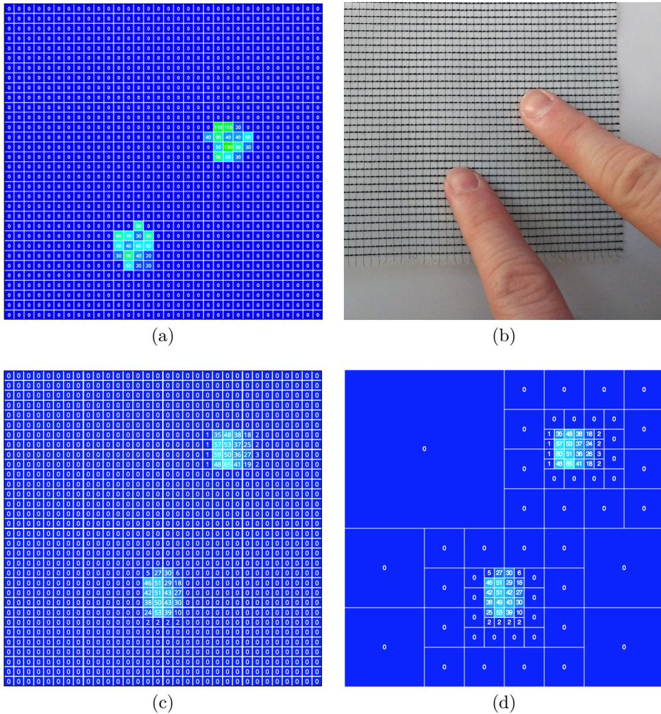
**Figure 7.11:** When the woven smart textile is touched with 2 fingers (b), two active areas are recognizable in the pressure pattern (a). The replication on the zebra fabric and the resulting quadtree structure are shown in (c) and (d), respectively.
