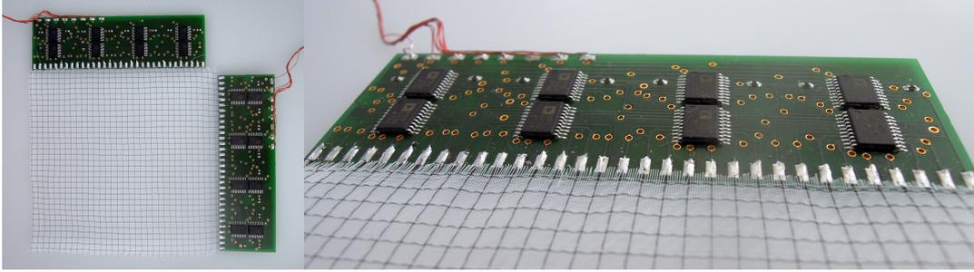
**Figure 6.6:** This is a prototype with an industrial woven smart fabric sensor with  $32 \times 32$  conductive yarns (black) which are connected to two boards with 8 analog matrix switches, respectively.
