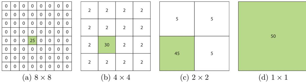
**Figure 6.10:** Without estimating the single sensor values, applied pressure is measurable in all resolutions.
