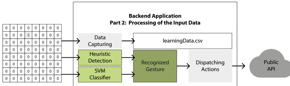
**Figure 4.15:** Two types of gesture recognition algorithms are performed on the input data once it is analyzed and filtered.
