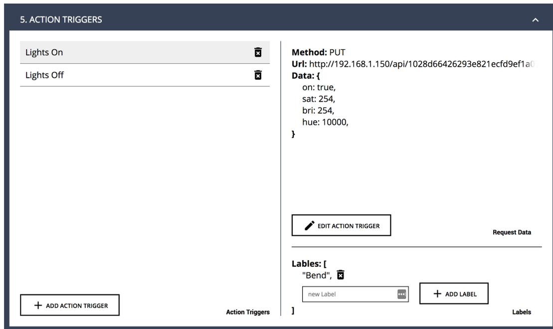
**Figure 5.6:** Section 5 is concerned with the definition of action triggers.
