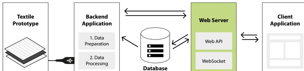
**Figure 4.18:** The web server handles the communication between the client and the backend application.
