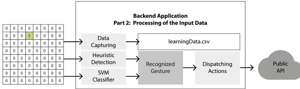
**Figure 3.3:** The input data is sent to the data capturing module and to the gesture recognition algorithms. If a gesture is detected and an action trigger for this gesture is defined, the corresponding HTTP request is dispatched.
