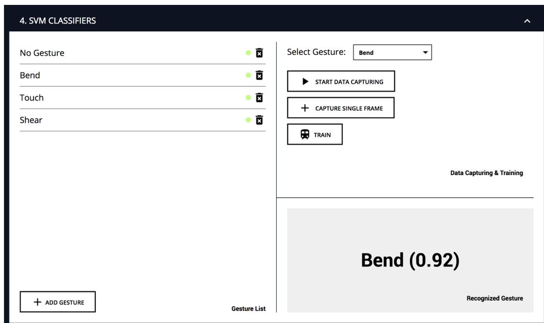
**Figure 5.5:** Section 4 is concerned with the definition of gestures and training of the machine learning algorithm. Gestures recognized by the SVM classifier are shown here.
