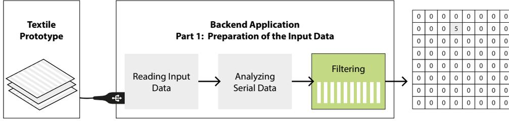
**Figure 4.4:** Once the analysis of the input data is complete, filtering is applied on the data to account for errors in the raw data.
