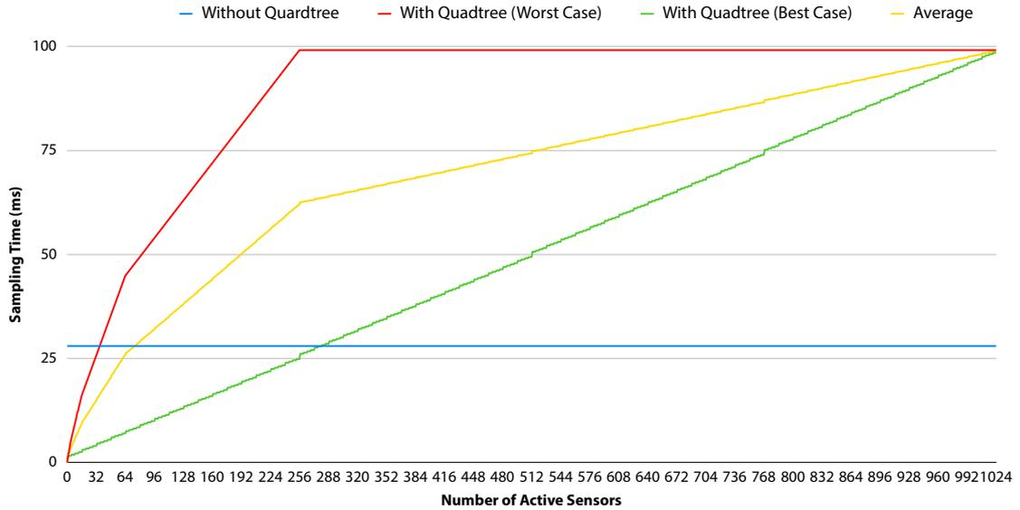
**Figure 7.6:** The performance of the quadtree approach depends on the number of active sensors. Without using a quadtree, the sampling of a  $32 \times 32$  sensor always takes 28 ms.
