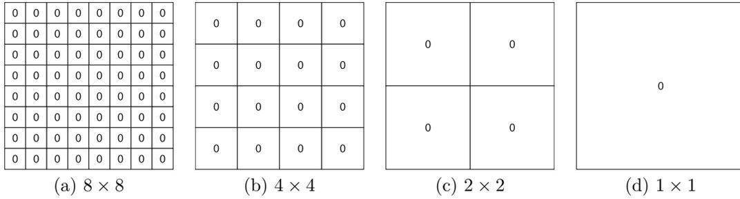
**Figure 6.8:** If the values of the single sensors are estimated and used as the value for the whole region, the result for a sensor where no pressure is applied is always 0 independent of the size of the sampled region.
