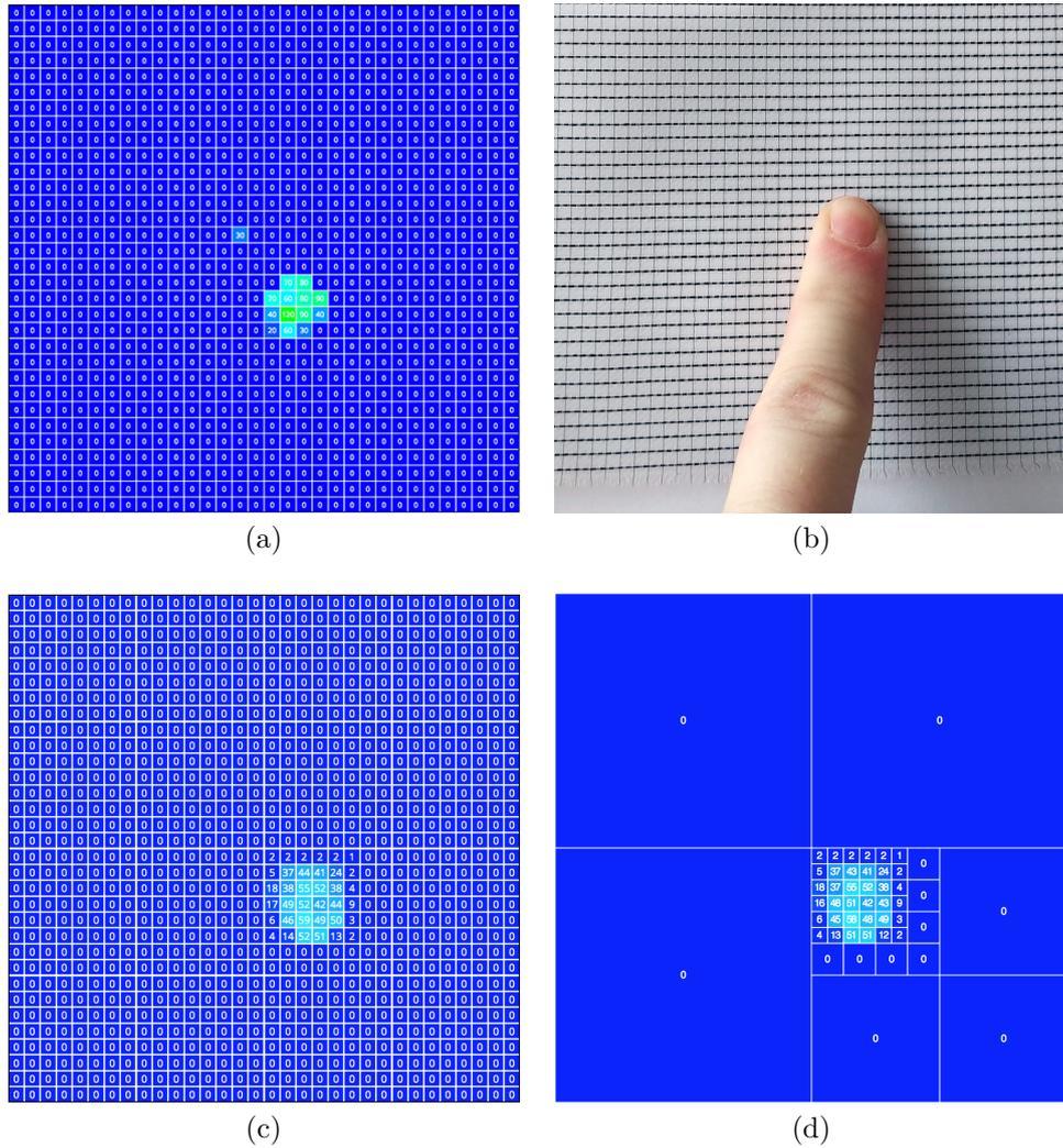
**Figure 7.10:** This figure shows the pressure pattern (a) of touching the smart textile with 1 finger (b). Again the sensor data was replicated on the prototype made out of zebra fabric (c) and the corresponding quadtree structure (d) is shown.
