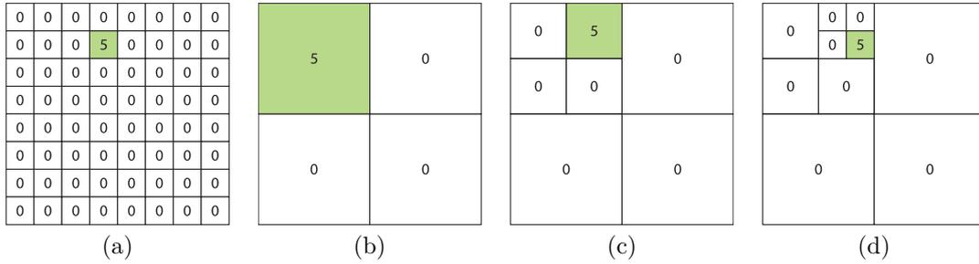
**Figure 6.2:** Instead of sampling all single sensors (a), the textile is divided in 4 parts (b) and only areas with a value above the threshold  $t$  are sampled in more detail (c). This step is repeated until the maximum resolution is reached (d).
