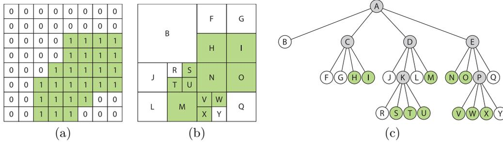
**Figure 6.1:** This figure shows an example for a *region quadtree* which was re-illustrated from [24]. The raw data (a) and the structured data (b) as well as the corresponding tree structure (c) are shown.
