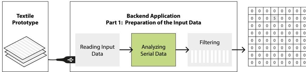
**Figure 4.2:** After the input data is read from the connected prototype, the data has to be transformed in the required data structure.
