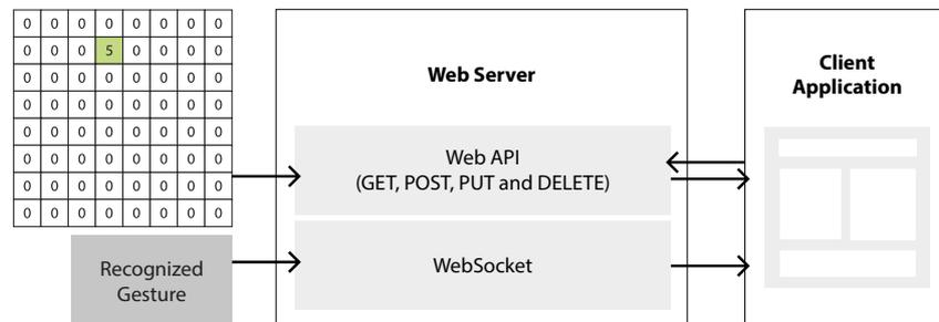
**Figure 3.4:** The sensor data and recognized gestures are sent to the user interface and visualized there. For the transmission the WebSocket connection handled by the web server is used. The user interface also communicates via the web API provided by the same server to interact with the backend application (see also Figure 3.1).
