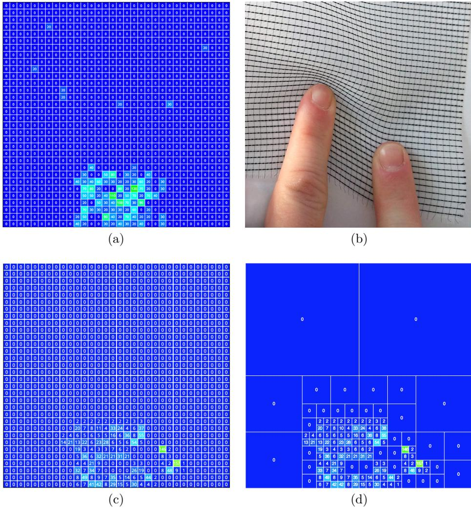
**Figure 7.13:** The pressure pattern (a) of a performed shear gesture (b) was replicated on the new prototype (c) and resulted in the quadtree structure shown in (d).
