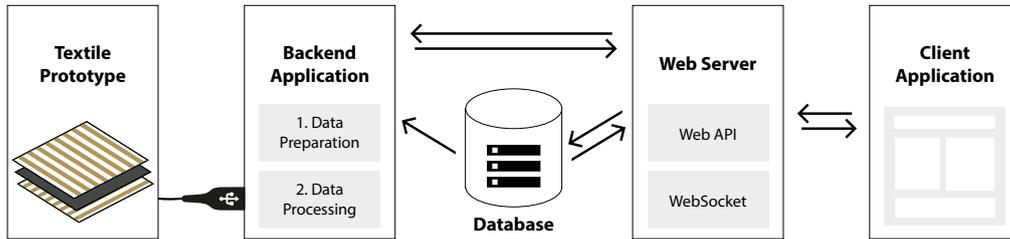
**Figure 3.1:** The application consists of a backend and a client part and a web server which handles the communication between them. Additionally, data is stored in a database to ensure consistency.
