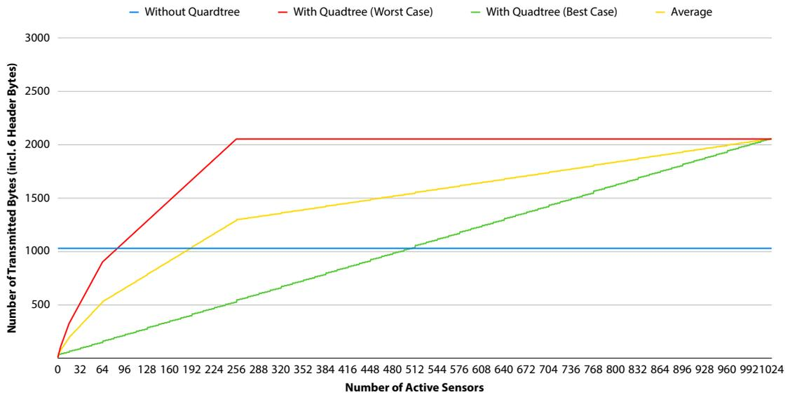
**Figure 7.7:** The transmitted quadtree data varies according to the number of active sensors. Without the quadtree method 1030 bytes are transmitted constantly.
