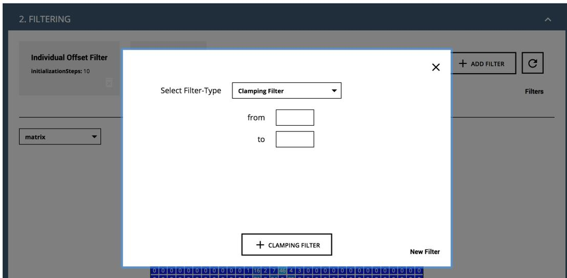
**Figure 5.3:** A modal containing a form allows to add new filters to the filter pipeline. The form fields change according to the selected filter type.
