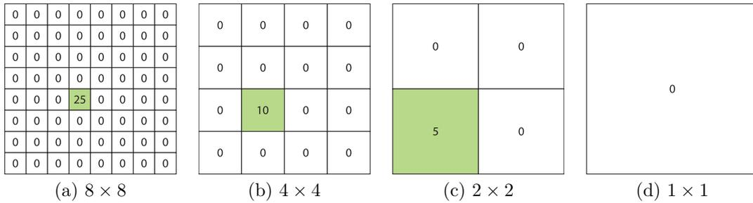
**Figure 6.9:** With increasing size of the sampled regions, pressure on selected sensors (a) has less input on the final value (b) and (c) until the pressure is not measurable anymore (d).
