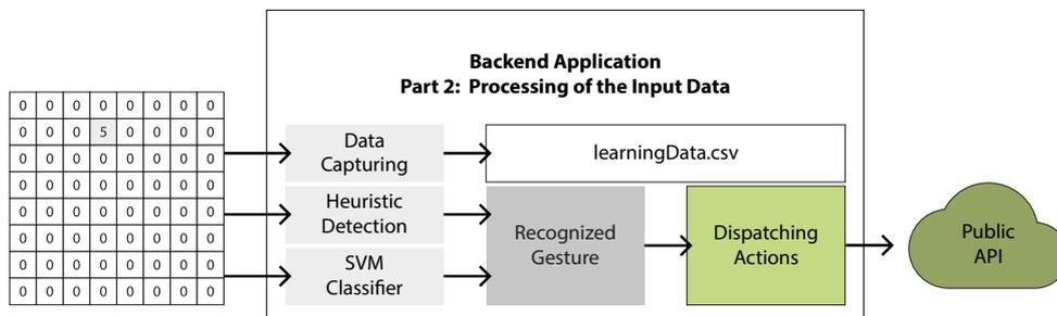
**Figure 4.17:** When a gesture is recognized, the configured action is dispatched which triggers a HTTP request to a public or custom API.
