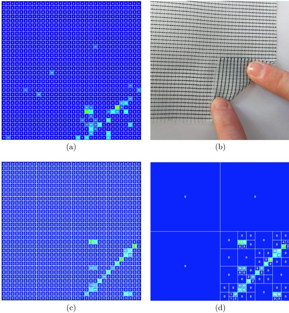
**Figure 7.8:** A fold gesture (b) was performed with the woven smart textile prototype, which resulted in the pressure pattern shown in (a). The sensor data was replicated on the new prototype (c) and resulted in the quadtree structure shown in (d).
