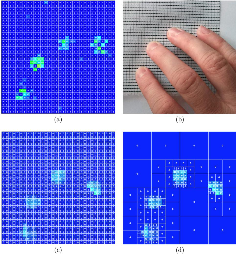
**Figure 7.12:** The pressure pattern for touching the smart textile with 4 fingers (b) is shown in (a). The pattern was then replicated on the prototype made out of zebra fabric (c). The corresponding quadtree structure is shown in (d).
