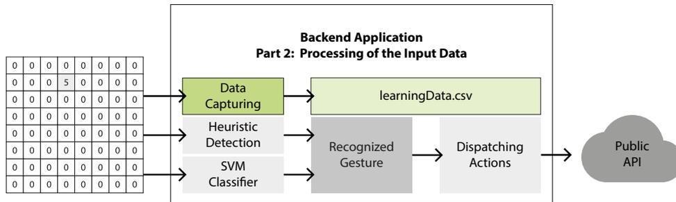
**Figure 4.16:** The prepared input data is passed to a data capturing module which stores the captured data to a specified CSV file.
