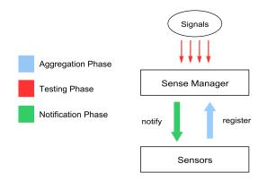
Figure 4.7: The different phases of the sense manager.
