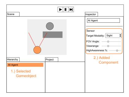
**Figure 4.3:** A sketch of the Unity UI showing the intended workflow of the sensory system implementation.
