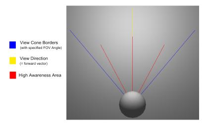
Figure 4.4: Screenshot of an agent with a sight sensor, showing its visual aid in the scene view.
