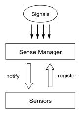
Figure 3.7: Basic functionality of a sense manager.
