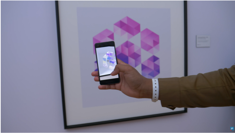
Figure 2.2: ARCore supports image recognition since version 1.2. Desired images are defined in a database. On recognition, a linked action is performed and the coordinates related to the origin can be used for further references [12].
