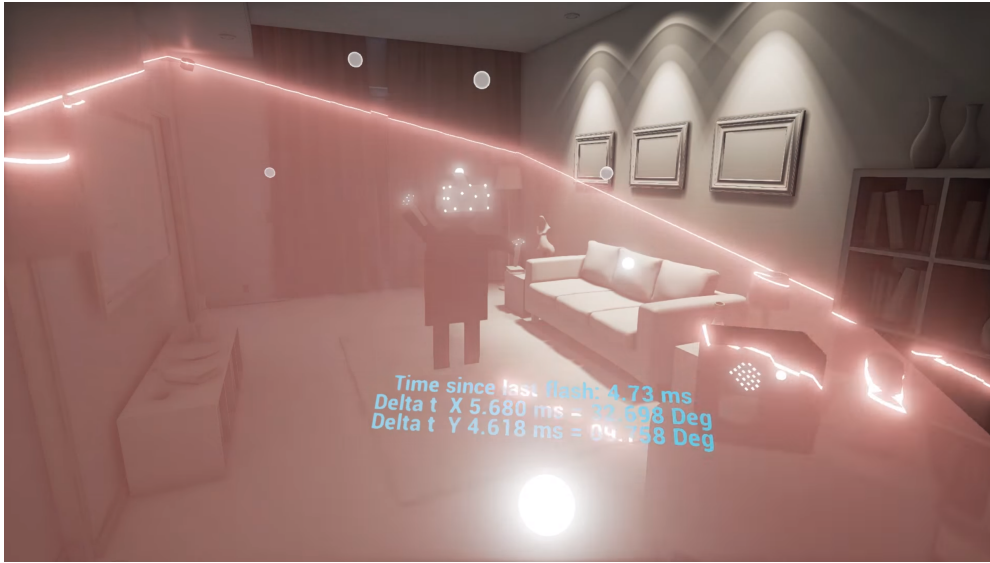
Figure 5.1: The tracking of SteamVR by HTC and Valve works with moving laser planes emitted by lighthouses . Depending on the timing of laser hits on the sensors, the position of a sensor in the room can be calculated. Using multiple sensors on a tracking device, such as the HTC Vive trackers , allow orientation tracking as well [14].
