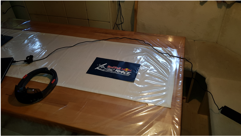
Figure 5.3: The reality setup of the spatial referencing is sticking a 30 by 16 centimeter big Red Bull Air Race logo flat on the tabletop. Evaluations in section 6.2.2 showed that a vertical alignment would be increasing the detection range but a horizontal orientation is for test cases easier to recreate.
