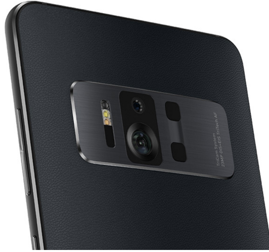
Figure 2.1: Devices which support Project Tango , such as the shown Asus ZenFone AR , require a wide variety of visual and emitting sensors to gather enough data of the three-dimensional surrounding [6].
