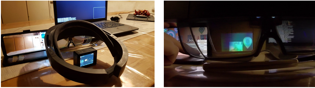
Figure 6.1: The activation on the instructor device ( Samsung Galaxy S8 ), receipt on the server (laptop) and remote activation of the pin on the HoloLens are recorded using an action cam with 120 frames per second to be independent of the device's timestamps.
